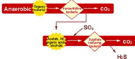
corrosiveness, the growth of filamentous sulfur bacteria, toxicity, etc. Aeration oxidizes H<sub>2</sub>S to odorless sulfur species, generating either free sulfur or sulfate. pH modification establishes basic pH conditions (7.5 – 8.0) so that the majority of the sulfide occurs in the odorless hydrosulfide ion form (HS<sup>-</sup>).
