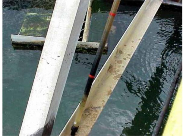
If there are too many solids in the bed there may be inconsistencies in the bed measurement. This makes it hard for a consistent RAS to be drawn off the bottoms, which impacts the returns of biosolids to the aeration basins. Holding solids in the clarifier too long generates systems conducive to filamentous growth or floating sludge or foaming, as the air, nutrients and proper conditions for growth are changed.
