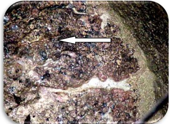
These have been called "Floating Turtles"- Hard solid formations that float around in the lift station. These can interfere with the pumps and can clog the pipes. Sometimes using a liquid product to spray on these can help reduce their size and shrink them faster.
