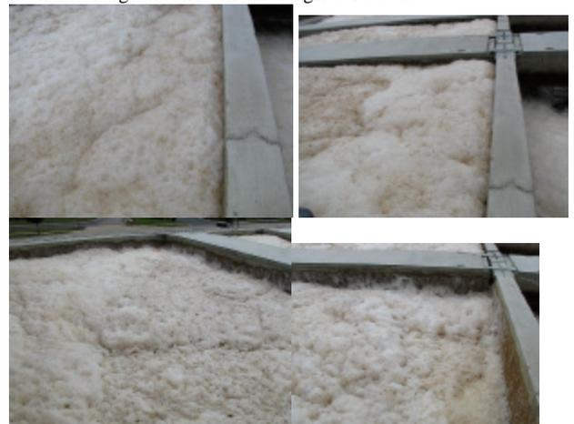
These 4 photos show a plant with serious foaming. The foam was almost up and over the edge in the top two. After topical addition of antifoam, you can see it dropped the foam 8-10 inches instantly.
