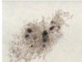
400x Dark anaerobic spots indicating septicity and low DO somewhere in the system, very different from carbon particles
