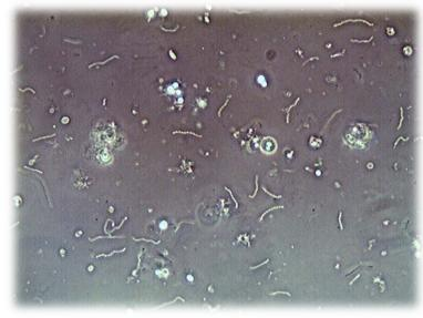
Many times antifoams are used when foaming occurs. Antifoams can be oil based and cause not only higher organic loading, but Free floating filaments or Nocardia or Zooglea due to oils. Antifoams can have a BOD of 2-700,000 ppm BOD. Nutrient deficiency can occur as well. Fix the issue instead of using band-aid
