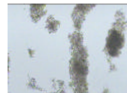
Irregular shaped floc 100x due to over addition of ferric
