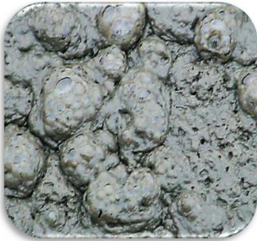
Foam due to Zooglea - High BOD & low nutrients Up & Right image Foam due to Nocardia - oils and grease Left down, Foam due to M. parvicella – grease Right down, Foam du to septicity & 0914.
