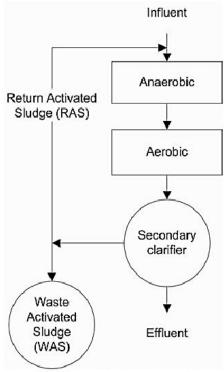
Figure 2. Anaerobic/Aerobic EBPR Process
