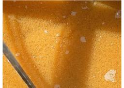
coalesce aluminum hydroxide solids is sometimes effective. At pH greater than 7, an anionic flocculant can be effective.
