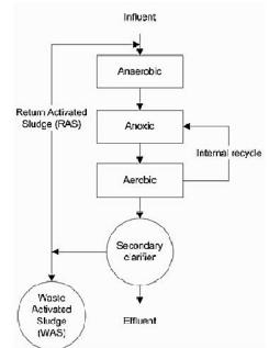
Figure 3. Anaerobic/Anoxic/Aerobic Process
