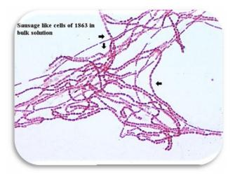
Wait; there also can be **Free floating filaments**. These can cause TSS problems. They can cause floating sludge and make it easier to violate a permit.
