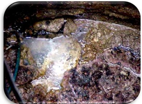
White milky water indicating bacteria is starting to work, cracks are starting to form in the grease; it is starting to soften and a little foaming is present.
