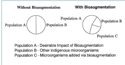
Figure 5: Conceptual Impact of Bioaugmentation on Bacterial Population in an Activated Sludge System
